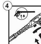
Insert high pressure hose into trigger handle.
