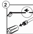
Assemble pressure washer gun to spray wand.
