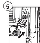
Connect the high pressure hose to the water outlet connector.
