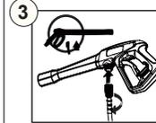
Insert high pressure hose into trigger handle.
