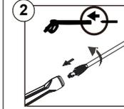
Assemble pressure washer gun to spray wand.
