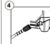
Insert high pressure hose into the pressure washer.
